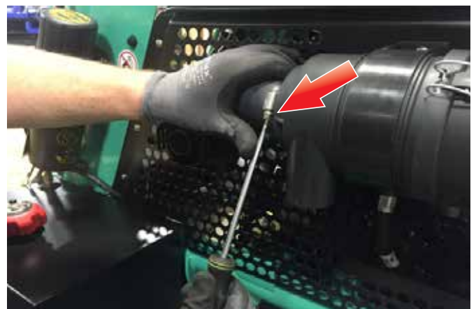
Figure 34. Reinstall Air Filter Intake Hose
