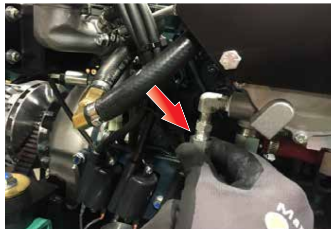
Figure 29. Connect Hose to Fitting
