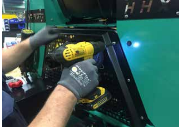
Figure 9. Rear Panel Removal
