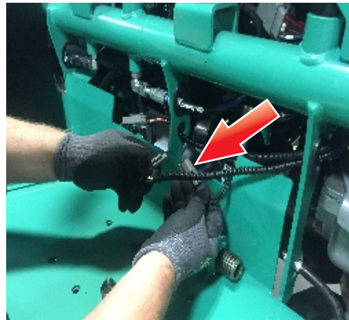
Figure 20. Unplugging Safety Lock Connector
