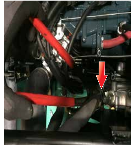
Figure 14. Crimping Stepless Clamps
