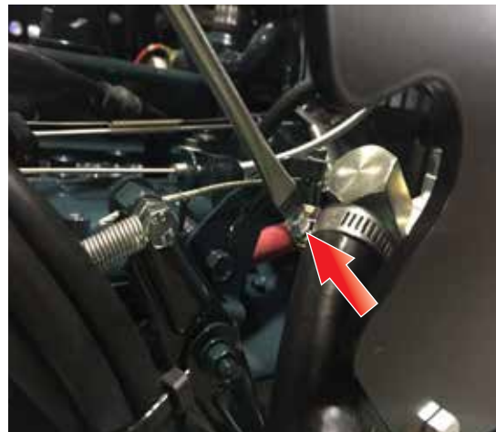
Figure 10. Loosen Hose Clamps
